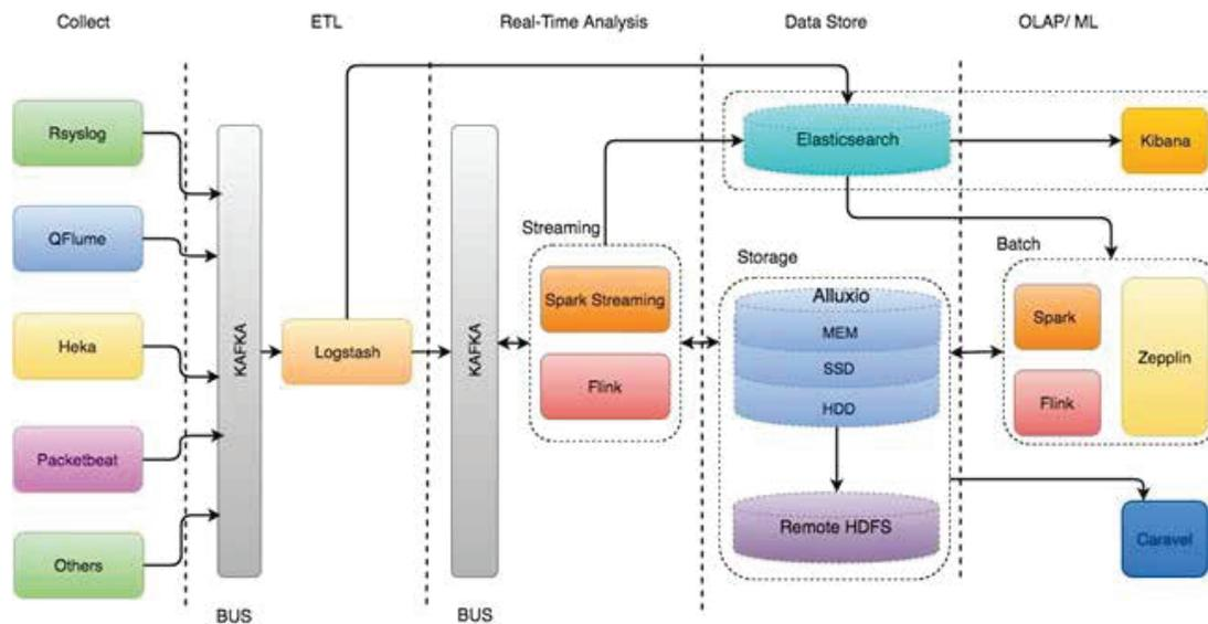
Much of the architecture is similar as before. The main difference is that much of the data used and generated by Spark streaming is stored in Alluxio, which avoids communication with the slow remote HDFS cluster. Meanwhile, the data stored in Alluxio can be conveniently shared by all the computing frameworks like Flink and Zeppelin. The following important Alluxio features played critical roles in improving the system's performance:
