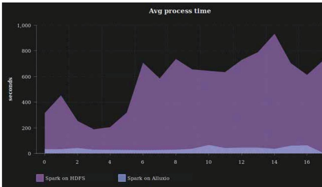
The overall throughput of the system also improves significantly. Below is a figure showing the throughput of the events consumed from Kafka. The previous architecture would process around 200K events/second, but with Alluxio the throughput reaches 1,200K events/second.
